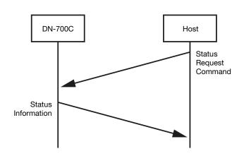
3. Status information automatically sent to the host when a change is made from DN-700C
