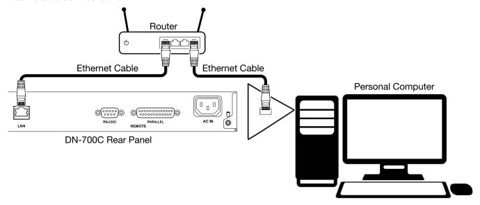
**Note:** Only one network user can be connected to DN-700C at a time. This means that two different computers cannot be used for serial communication with DN-700C at the same time, and you cannot use the LAN port for serial communication while DN-700C is already being controlled by the web browser remote.
